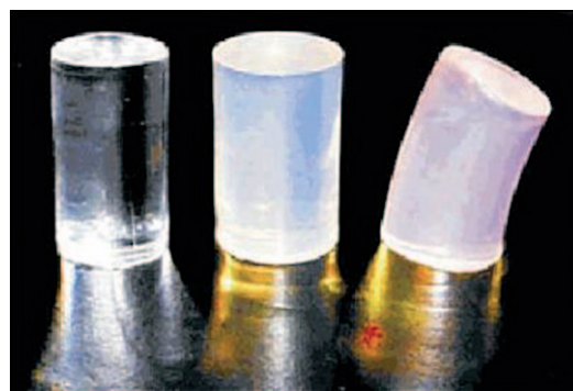
Figure 5. Hard and rubbery materials formed by polymerization under the same conditions: pure polystyrene (left); gel-derived polystyrene using 1 wt% DRC (middle); and gel-derived poly(2-ethylhexylmethacrylate) using 1 wt% DRC (right). The rubbery material (right) was mechanically deformed by hand before the image was taken. [61]
